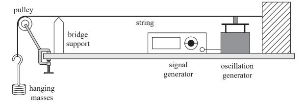
When the signal generator was switched on the string oscillated. The signal generator was adjusted until the string resonated.
