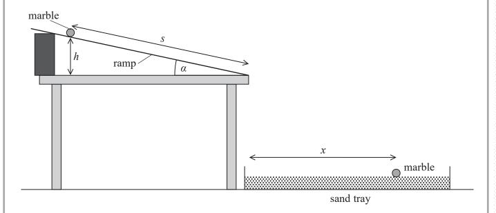
Some students investigate how the horizontal distance x the marble travels between the end of the ramp and where it lands in the sand tray is related to the angle of the ramp  $\alpha$ .
