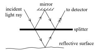
An incident light ray is directed at a splitter. The splitter partially reflects and partially transmits the ray. The reflected ray then hits a mirror and is reflected back to the splitter. The transmitted ray hits the reflective surface and reflects back to the splitter. The two rays then travel to a detector where superposition occurs.
