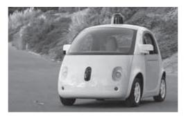
The new car contains systems to detect other vehicles. One system uses a pulse-echo technique with laser light and another system uses the Doppler effect with microwaves.
