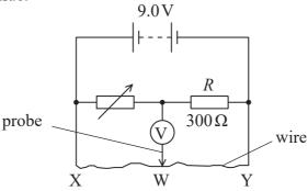
(i) The student moved the probe attached to the voltmeter along the wire until, at W, the reading on the voltmeter was 0 V. This occurred when the length XW was 33.0 cm.
