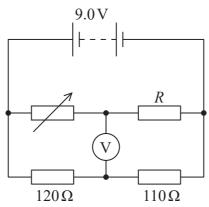
As the student adjusted the variable resistor, the reading on the voltmeter changed. When the variable resistor had a resistance of  $295\,\Omega$ , the reading on the voltmeter was 0 V. This happened because the p.d. across the variable resistor was equal to the p.d. across the  $120\,\Omega$  resistor.
