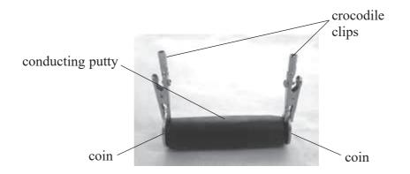
(a) The student made a cylinder of conducting putty of length 0.075 m and diameter 9.0 mm.
