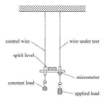
Every time a known weight was added to the applied load the micrometer was adjusted until the spirit level was horizontal. The movement of the applied load was the same as the movement of the micrometer.
