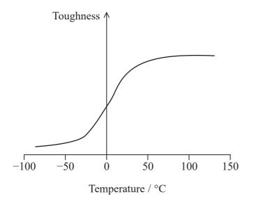
The brittleness and malleability of the steel also vary with temperature.
