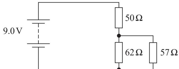
Calculate the total resistance of the circuit.
