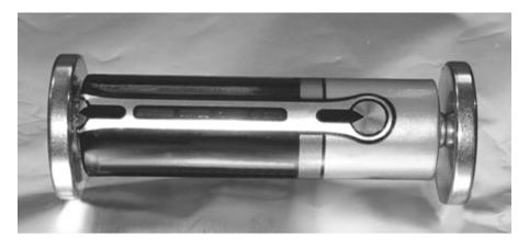
When the motor is placed on an aluminium sheet, the motor begins to roll.
