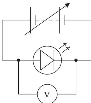
He increased the potential difference  $V$  from zero and recorded the value at which the LED just began to emit light. He repeated this for LEDs that emitted light of different, known frequencies  $f$ .
