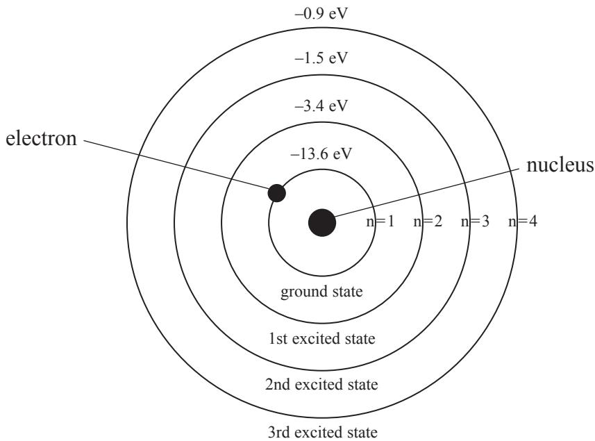
In this model an electron can orbit the nucleus at different energy levels, some of which are shown in the diagram.
