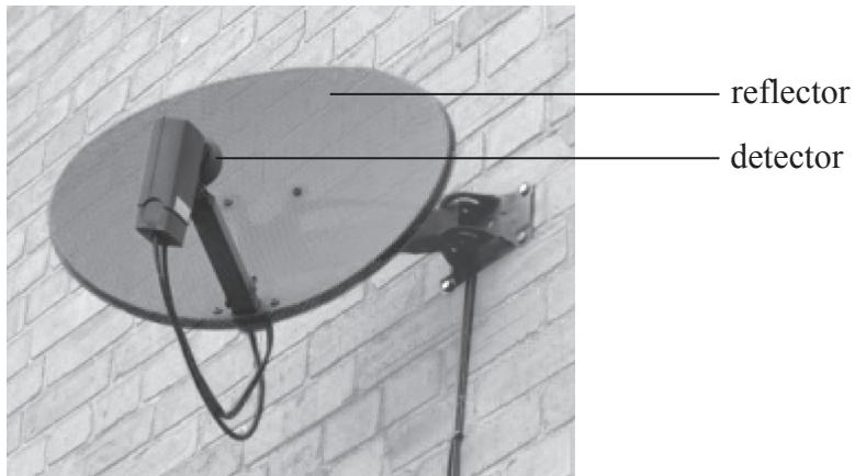
Electromagnetic radiation from a communications satellite is reflected from the reflector to the detector.
