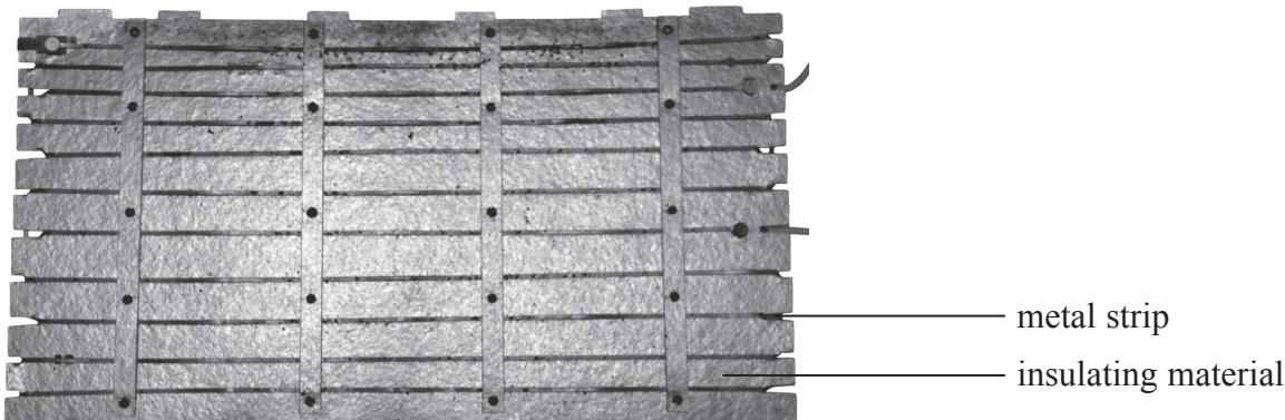
The metal strip carries a large current producing a high temperature. As a result, infrared radiation is emitted which toasts bread.
