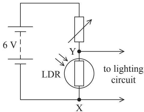
The resistance of the LDR decreases as the radiation flux of the incident light increases.
