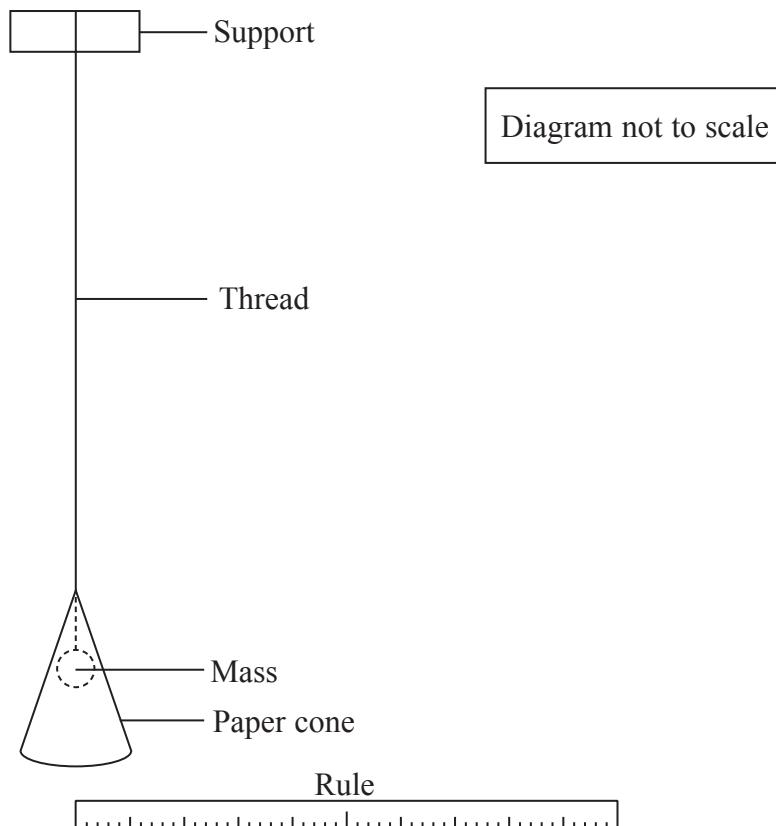
(a) The pendulum is pulled to one side and released so that it oscillates. The amplitude of oscillation decreases because the cone provides damping.
