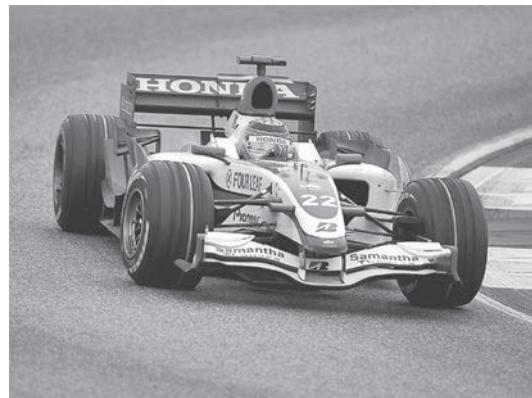
Racing cars have to go through large changes in speed in order to go around the corners on the racing tracks. All racing cars have a kinetic energy recovery system which recovers the moving vehicle's kinetic energy when it is braking. The recovered energy can now be stored in ultracapacitors for later use when the car is accelerating.
