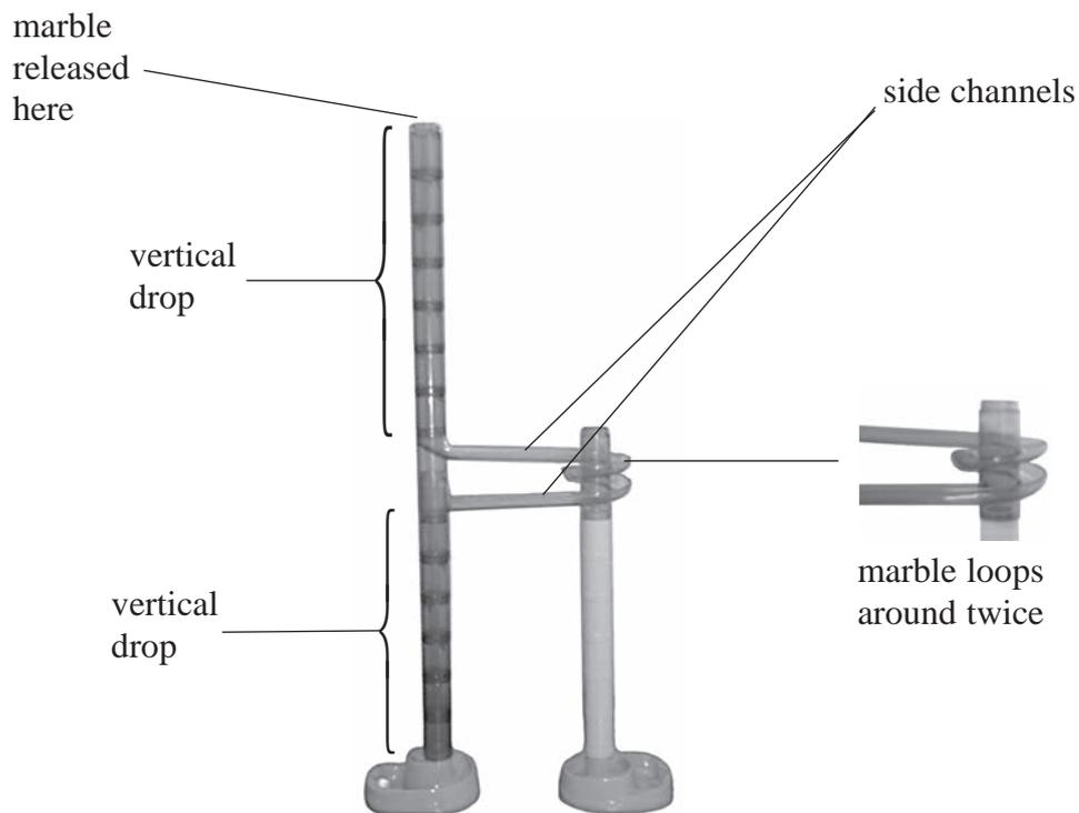
A marble was released and its motion was recorded using a digital video camera. The data was uploaded to a computer and then analysed using a motion capture programme. The following vertical displacement-time graph was obtained.
