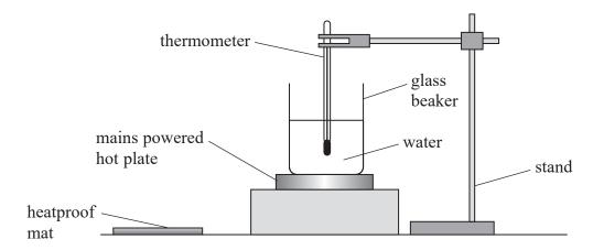
(a) The student used the hot plate to heat the water until it boiled.
