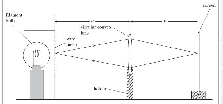
The student moved the position of the holder until the lens formed a sharp image of the wire mesh on the screen. She measured the distances u and v with a metre rule.
