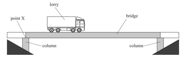
Forces P and Q act on the bridge from the columns. The centre of gravity of the bridge is at its centre. At a particular time the lorry is  $35 \,\mathrm{m}$  from point X.
