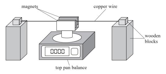
The student connected the copper wire to a circuit which included a power supply with a fixed potential difference. The maximum current from the power supply was 5 A.
