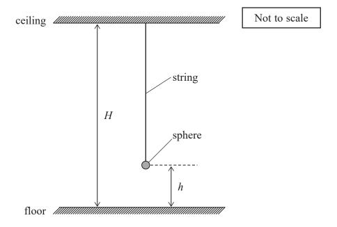
The student displaced the sphere through a small angle, so that it oscillated. She determined the time period T when the centre of the sphere was a distance h from the floor.
