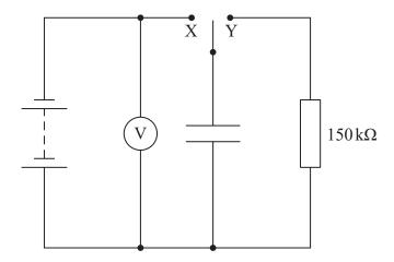
The student connected the switch to X to charge the capacitor. She then connected the switch to Y so that the capacitor discharged through the  $150\,\mathrm{k}\Omega$  resistor.
