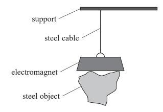
(i) When the object is suspended, the strain in the cable is  $3.0 \times 10^{-4}$
