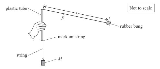
The rubber bung with mass m was rotated around the plastic tube at a constant angular velocity  $\omega$ . The part of the string between the rubber bung and the plastic tube was almost horizontal.
