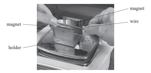
\*(a) When the student moved the wire quickly downwards between the magnets, the reading on the balance changed.
