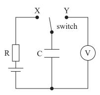
The student planned to use the circuit to measure the potential difference V across the capacitor C as it was charged and discharged through the resistor R.
