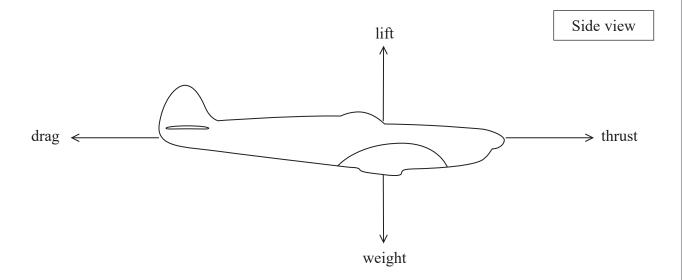
(a) The lift force is perpendicular to the wings.
