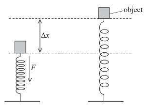
When  $\Delta x$  becomes zero the object has a vertical speed v.
