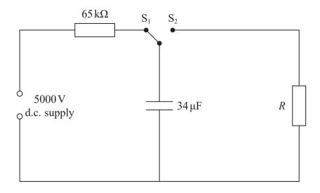
(a) When the capacitor is completely discharged, the two-way switch is moved to position  $S_1$  at time t = 0 s.
