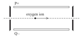
(i) A uniform electric field between the plates acts on an oxygen ion. A uniform magnetic field acts so that the magnetic force on the oxygen ion is in the opposite direction to the electric force.
