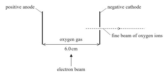
(i) The electric field strength between the anode and cathode is  $7.5 \times 10^5 \, \mathrm{V} \, \mathrm{m}^{-1}$ .
