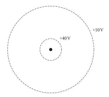
(i) Sketch lines to show the electric field between these two lines of equipotential.
