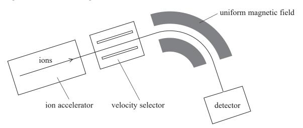
(a) An ion accelerator uses an electron beam to ionise atoms of oxygen gas. The positive ions are then accelerated across a high potential difference between an anode and a cathode, as shown in the diagram below. The cathode has a hole in it so that the accelerated ions may pass in a fine beam to the velocity selector.
