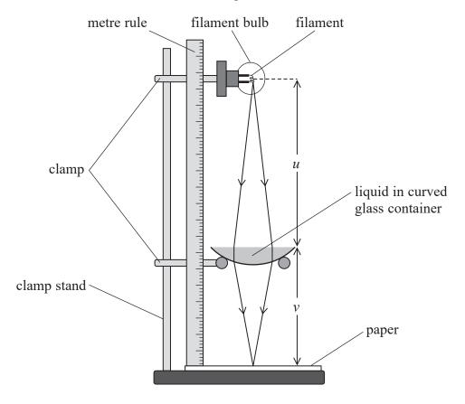
The student adjusted the position of the filament bulb until a clear image of the filament was formed on the paper.
