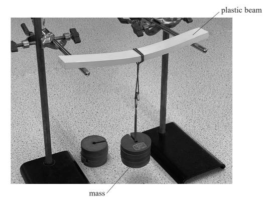
The beam bent downwards as shown.
