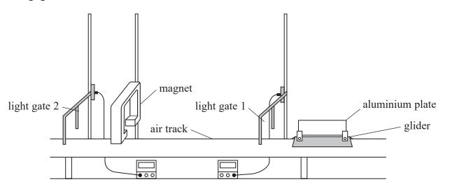
(a) (i) The vehicle was given a push. The aluminium plate took 0.19 s to pass through light gate 1.
