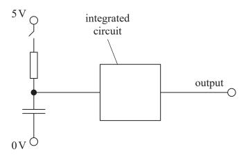
(a) (i) Sketch a graph to show how the potential difference  $V_{\rm C}$  across the capacitor varies with time t as the switch is closed. The time constant T for this circuit is marked on the time axis.
