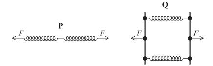
When one spring is subjected to a tensile force F, the elastic strain energy for the spring is E.
