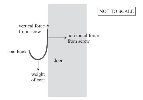
Add a labelled arrow to the diagram to show the additional force required for the coat hook to be in equilibrium.
