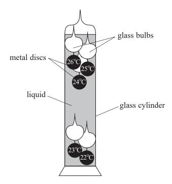
As the temperature increases, the density of the liquid decreases. This can cause the bulbs to move within the liquid.
