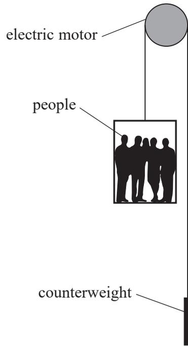
(a) Explain how the counterweight affects the amount of work required from the electric motor to raise the lift.
