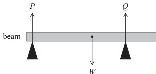
The beam has a weight  $W$  and the reaction forces at the two supports are  $P$  and  $Q$ .
