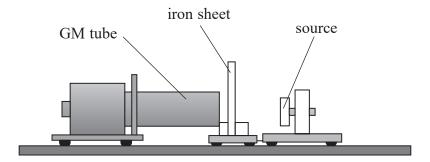
The student used five different thicknesses of iron and determined the count rate for each thickness.
