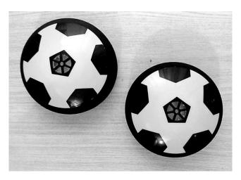
The pucks each contain a small fan, so that they glide across the table on a cushion of air. The mass of the pucks can be varied by attaching small masses.
