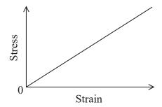
Show that the area under this graph represents the work done per unit volume in stretching the sample.
