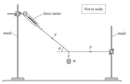
(a) The force meter allows force to be measured by means of Hooke's law.
