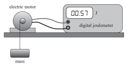
The students used a joulemeter to measure the energy supplied to the motor to lift a mass a distance of 75 cm. They repeated the experiment twice before increasing the mass.
