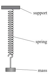
The mass is then displaced a further 3.5 cm vertically downwards and released. The mass oscillates with simple harmonic motion.
