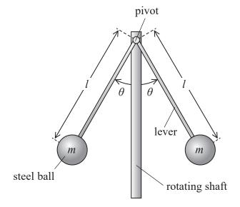
Two steel balls, each of mass m, can move apart at the end of levers that are freely pivoted. As the vertical shaft rotates, the two steel balls move apart so that the angle between the lever and the vertical is  $\theta$ .
