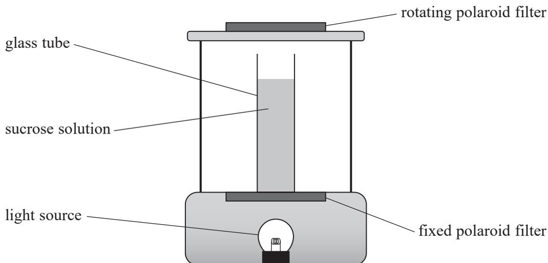
The angle of rotation depends on the concentration of the sucrose solution
