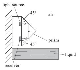
When the liquid is below the level of the prism the light totally internally reflects to the receiver as shown.
