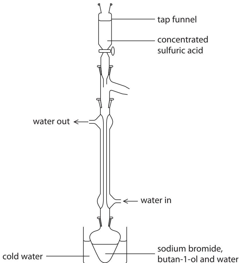
**Step 2** 10 cm<sup>3</sup> of concentrated sulfuric acid is dripped slowly from the tap funnel into the reaction mixture. The flask is shaken gently.
