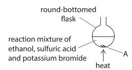
(e) Identify the solid particles labelled **A** in the flask that have been added to promote smooth boiling.
