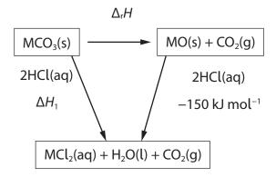
In an experiment to determine  $\Delta H_1$ , 0.050 mol of MCO<sub>3</sub> was placed in a 100 cm<sup>3</sup> beaker. 60 cm<sup>3</sup> of 2 mol dm<sup>-3</sup> hydrochloric acid (an excess) was added and the mixture stirred. The maximum temperature rise measured was 6.0 °C.
