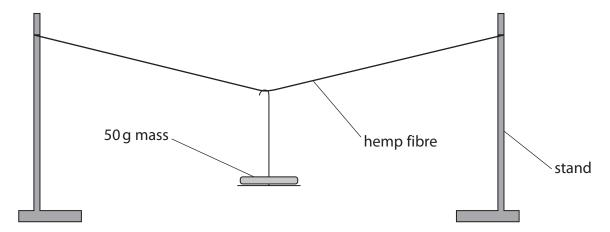
(i) Describe how you could use this apparatus to make a valid comparison of the tensile strength of fibres with different diameters.
