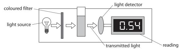
The transmission of light through the solution decreases as the intensity of the colour increases.
